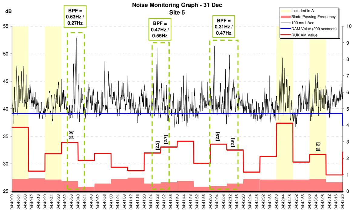
**Figure 2: Cotton Farm - 31 Dec - 04:40 - example of inconsistent RUK blade pass frequencies.**
