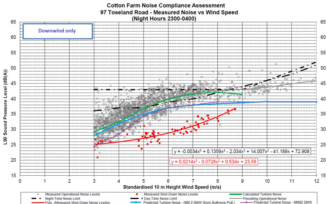
**Figure 1: Compliance measurements at Cotton Farm Wind Farm - predicted turbine LA90 v actual turbine LA90**
