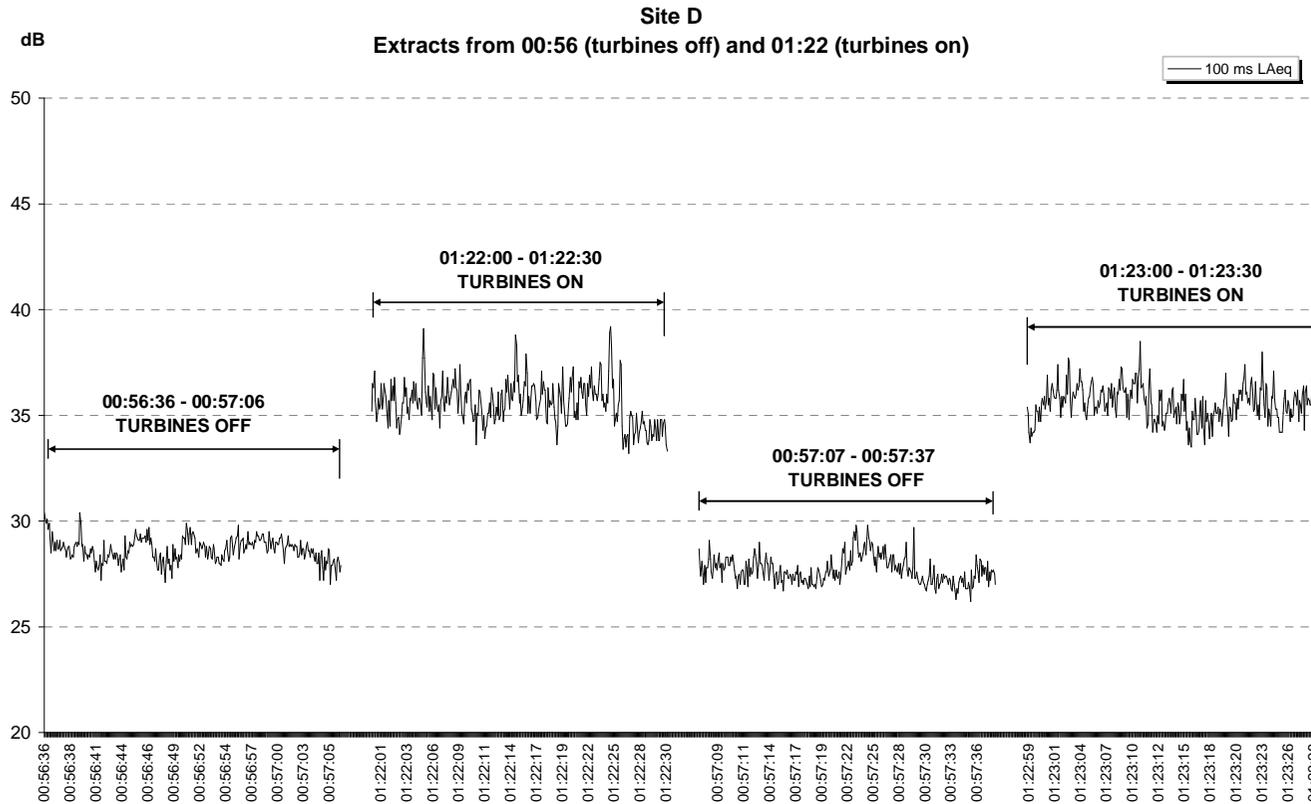
The measurements were made in an external amenity area location in a remote rural area approximately 1km from the wind farm. The graph compares a period when the turbines are not operating with a period just under half an hour later when the turbines are operating. There is approximately a 7dB increase in background noise level and the character of the sound scape is significantly altered.
