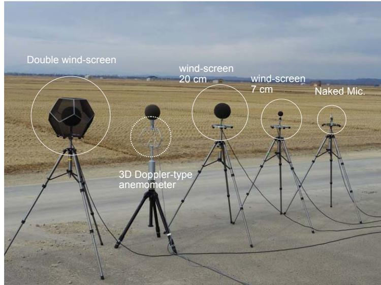
Figure 4: Experimental arrangement in the field measurement
